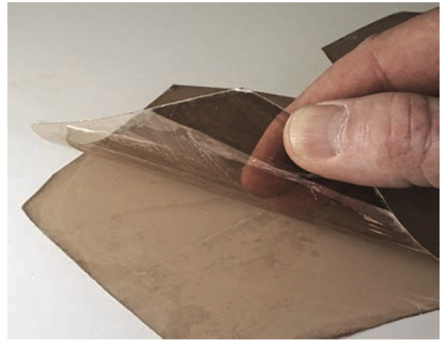
▲ Figure 1.22 Sheets of elastic minerals, like muscovite, can be bent but will snap back when the stress is released. Sheets of muscovite are transparent because they transmit both light and images. (Photo by Dennis Tasa)
